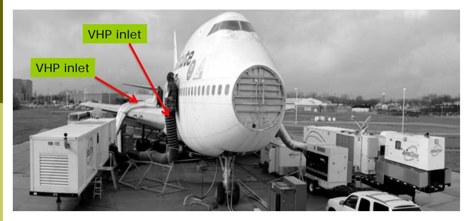
The first demonstration of whole widebody airliner VHP decontamination, March 2007, following on from a narrow body aircraft demonstration in 2006 (Air Transportation Center of Excellence for Airliner Cabin Environment Research, Auburn University, USA).
